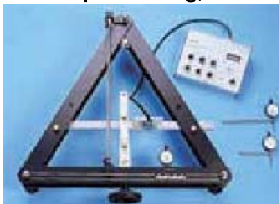
EX152 - EX154 specimens used with the EX150 Test Unit and connected to the EI 616 Strain Bridge
