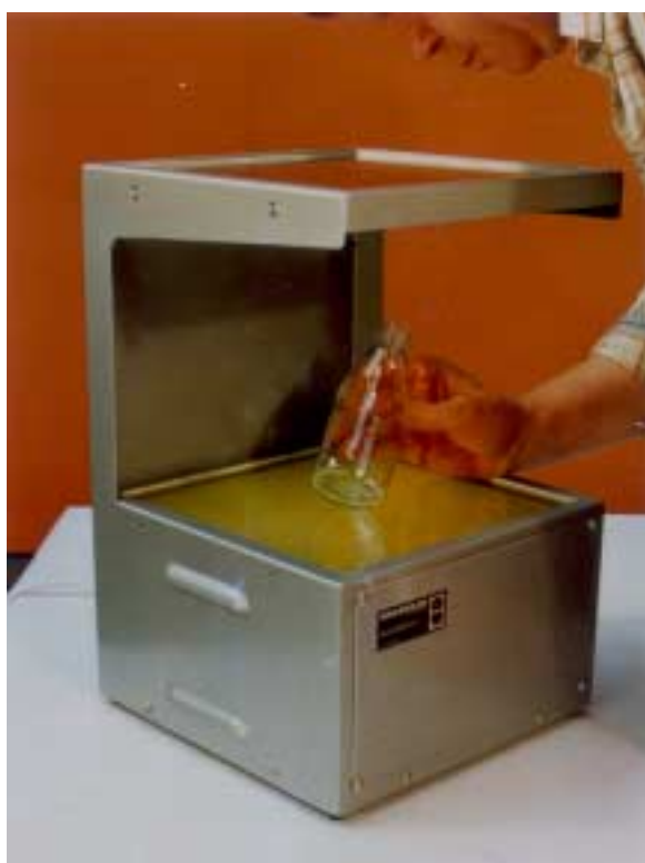
The General Purpose Strain Viewer being used in the vertical working position.
